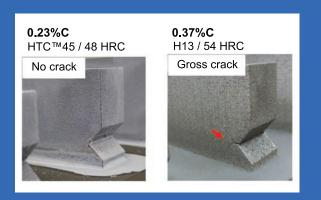
BOTH MATERIALS WHEN PRINTED PROPERLY HAVE A DENSITY OF 99.96% AND DUE TO THE POWDERS EXCELLENT FLOW RATE THE SURFACE FINISH IS SMOOTH AND CONSISTENT ENOUGH TO BE POLISHED WITH EASE.
